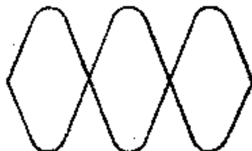
TWO TONE LINEARITY TEST OBTAINED WITH SINGLE TONE INPUT, WITH CARRIER BALANCED OUT ON AM
