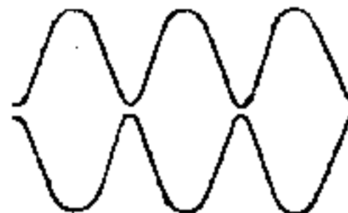
DOUBLE SIDEBAND AM WITH CARRIER 100% MODULATED
