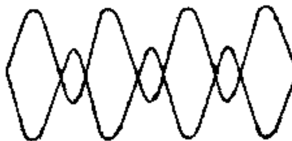
DERC DOUBLE SIDEBAND REDUCED CARRIER OBTAINED BY REDUCING CARRIER LEVEL AND INCREASING AUDIO INPUT LEVEL.
